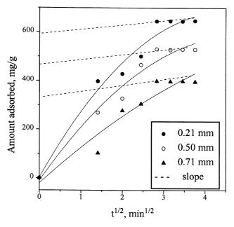
**Figure 8.** Intraparticle diffusion plot for the adsorption of Fe(III) on chitin at different particle sizes.
